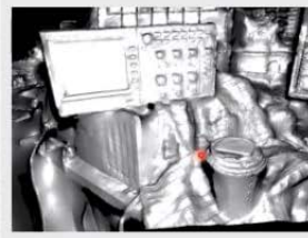
Dense Tracking and Mapping The dense map generated by the DTAM system. All points on the surface are part of the map
