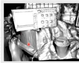
Dense Tracking and Mapping The dense map generated by the DTAM system. All points on the surface are part of the map
